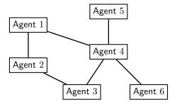
A node represents a computational agent that stores data and performs computation, and an edge  $\{i,j\}$  represents a direct connection between i and j through which agents i and j can communicate.
